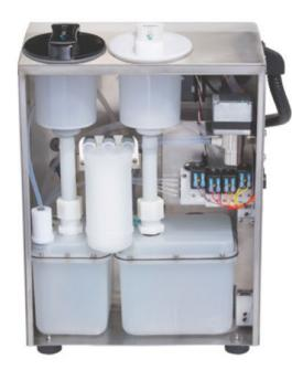
EcoTec<sup>™</sup> fluid management system reduces solvent consumption, lowering overall cost of ownership while extending the time between solvent additions and filter replacements.
