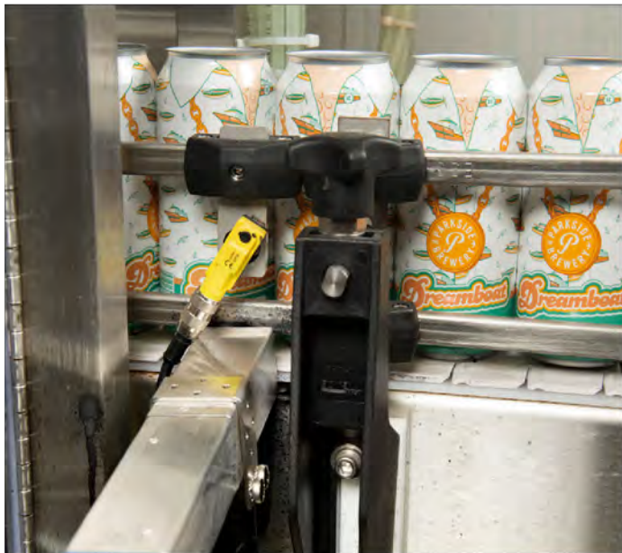
Featuring a CleanStart industrial stainless-steel printhead, the model 82 coder manufactured by BestCode and purchased by The Parkside Brewery through Weber Marking Systems, throws ink onto cans of beer for non-contact application at a rate of 196 meters per minute.
