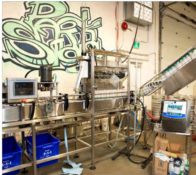
Along with the BestCode model 82 coding system from Weber Marking Systems, The Parkside Brewery also uses a micro-canning system designed and built by Calgary-based Cask Brewing Systems, which manufactures economical canning solutions designed for the need of small and mid-sized craft brewers.
